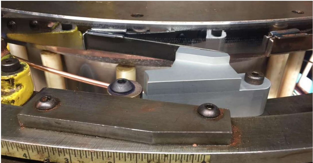
Figure 22. An overall view of the improved finger base and back-plate installed.
