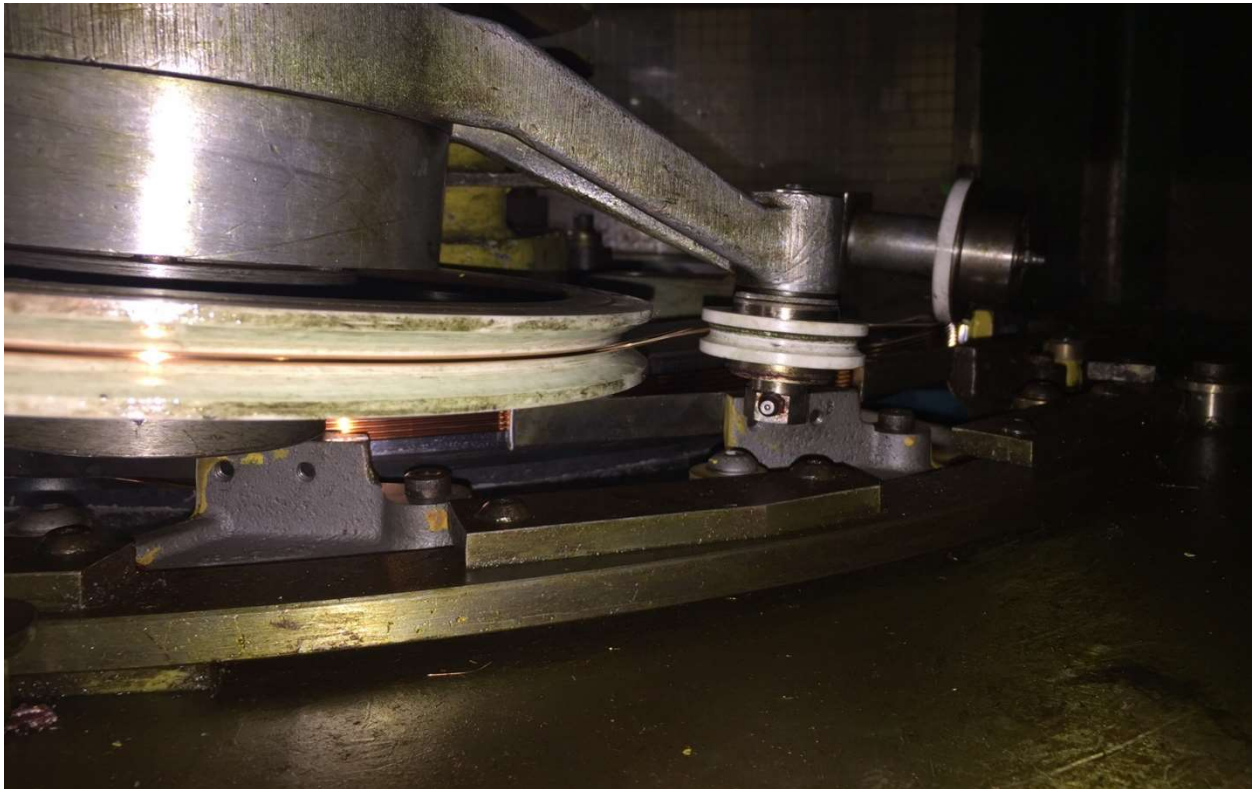
Figure 19. An image of the radial arm. The portion below the small white pulley is the cause of the damage to the finger base.
