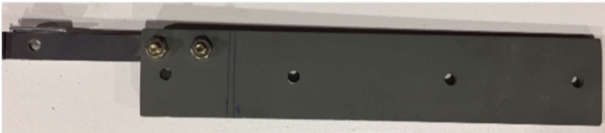
Figure 7. An image showing the finger with a hole drilled at the approximate point of contact (3/4 of an inch) and mounted to the flat steel stock.
