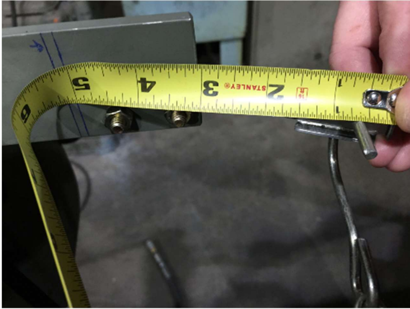
Figure 9. An image showing the change in dimension when loaded versus unloaded, matching the dimensions when the finger is installed in the machine.
