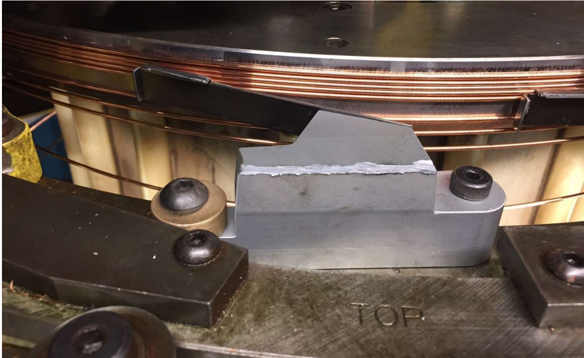
Figure 18. A close-up view of the damage done to the finger base.
