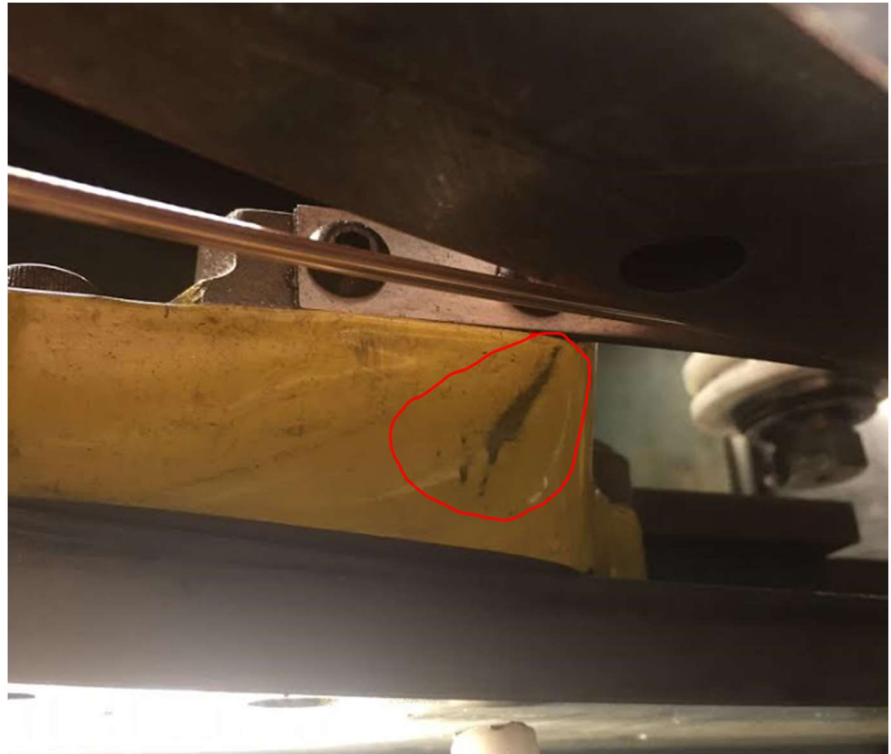
Figure 4. An image showing the exact contact location between the coiled wire and the finger base.
