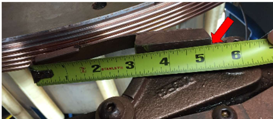
Figure 5. Shown here is an image of a finger that is mounted in the machine. The length from the tip of the finger to the back of the mounting block is approx. 5-5/32 inches.
