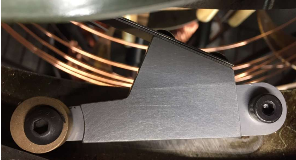
Figure 16. A top view of the finger base installed in the machine.
