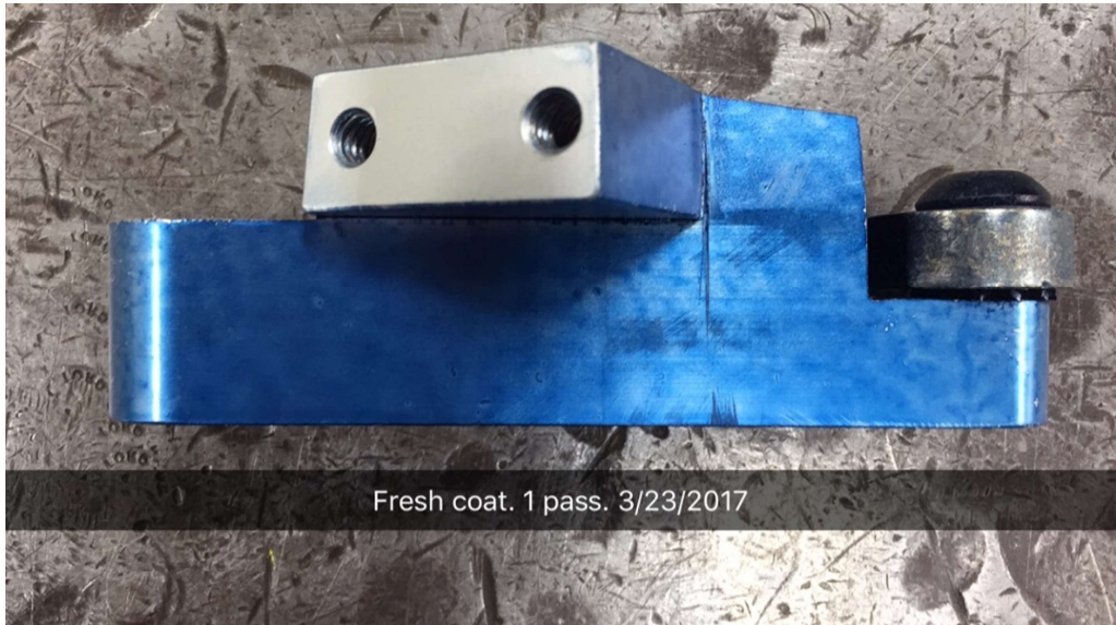
Figure 23. A view of the improved finger with a coat of layout fluid on the day it was installed to be tested in the coiler.
