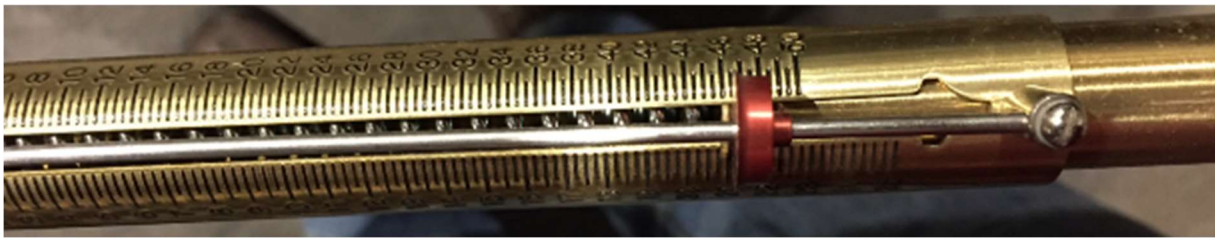
Figure 10. A close-up view of the force gauge. Reading is approx. 47 lbs.
